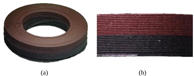
Figure 1: (a) toroidal NiZn-MnZn bi-material magnetic core; (b) Side view of the printed core.
