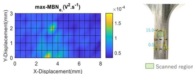
Figure 1: Right side: max(MBN) measurement, Left side: tested specimen.
