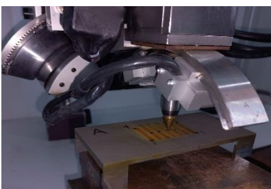
Figure 1: X-ray diffraction residual stress technique.
