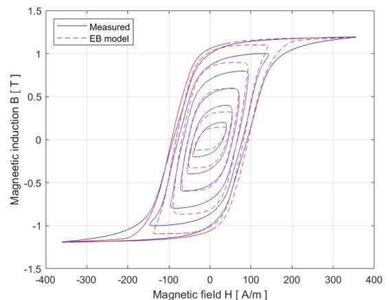
Figure 2: Comparison of the hysteresis cycles. Blue solid line: measured data. Red dashed line: EB simulated cycles.
