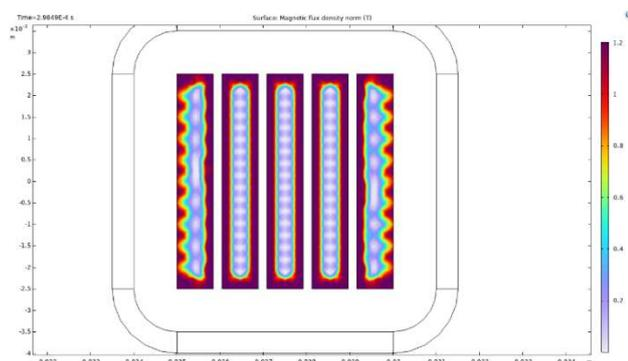
Figure 1: Distribution of the magnetic induction field  $B$  in Tesla at a given time step over a section of the sample.
