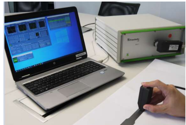
Figure 1: 3MA NDT system under test.
