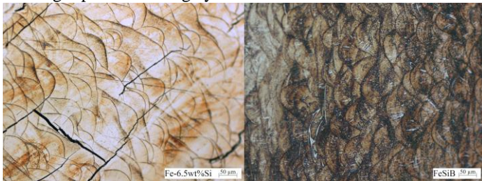
Figure 1: Optical microscopy image of Fe-6.5wt%Si (left) and FeSiB (right).
